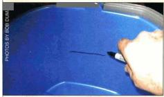
For a simple bucket test, use a waterproof marker to draw a line inside a clean, 5-gallon bucket.
