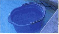
Place the partially filled bucket on the pool steps and note the water level on the outside of the bucket.
